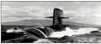
The USS Benjamin Franklin was built by the Electric Boat Division of General Dynamics Corporation in Groton, Connecticut and was launched on 5 December 1964. She was 129.54 meters (425 feet) in length and was powered by a S5W reactor and was the lead ship of her class of ballistic missile submarine.
